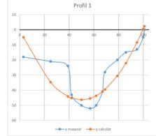
Fig. 4 Soil profile 1 – interpolation nodes measured vs. calculated
